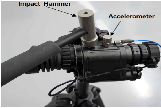
Fig. 9 Modal test for NVG housing
