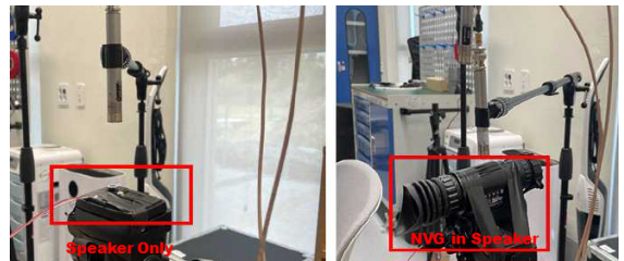
Fig. 8 Method for insertion loss test
