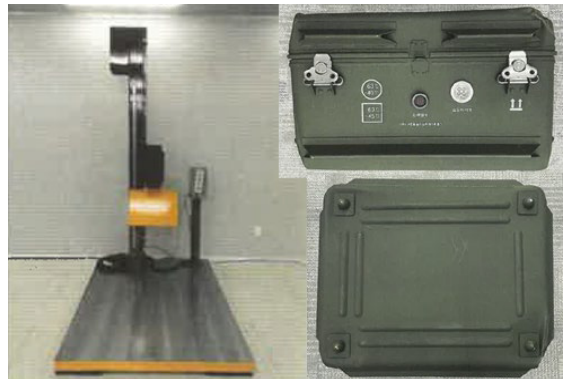
Fig. 6 Drop tester and test results
