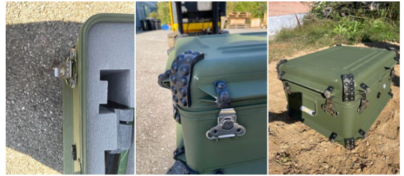
Fig. 17 Drop test results of IFF box
