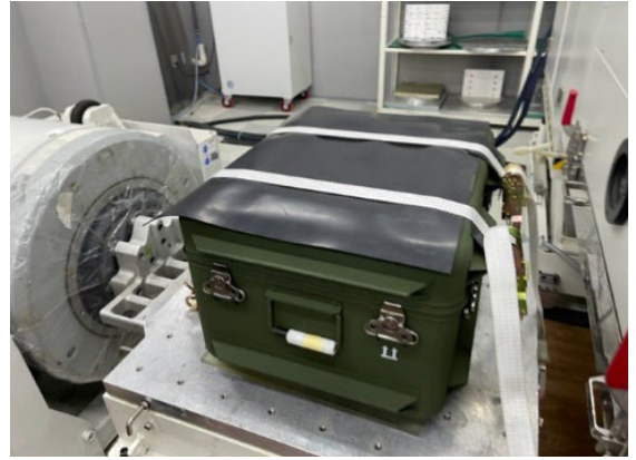
Fig. 4 Transport vibration test of IFF box
