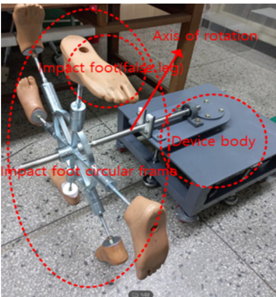
Fig. 2 Manufactured continuity impact source prototype
