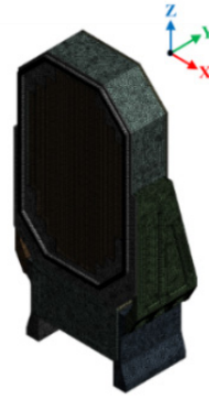
Fig. 2 Finite element model of antenna structure
