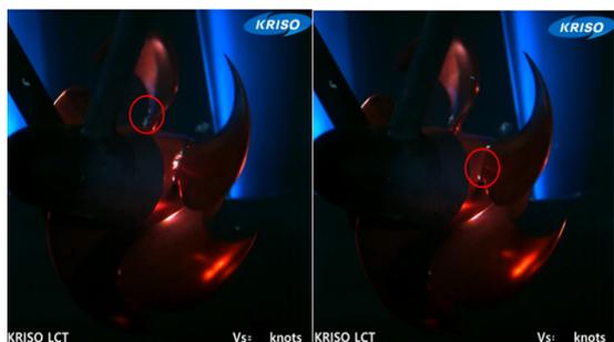
Fig. 74 Root cavitation occurrence and collapse
