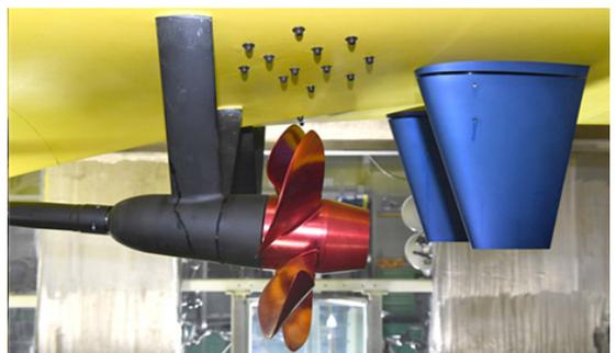
Fig. 4 Test setup for model ship of large cavitation tunnel
