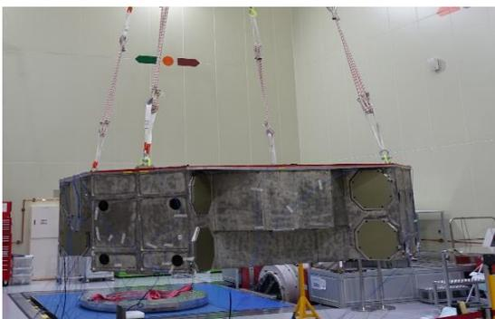
Fig. 15 Modal test configuration on head-expander
