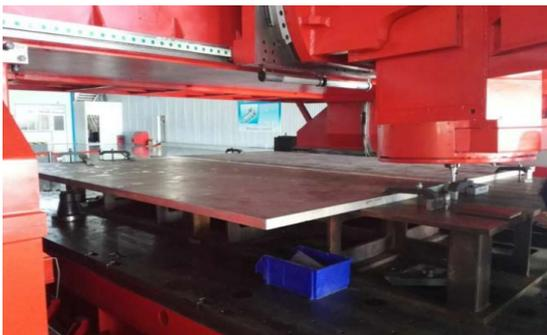
Fig. 10 FSW on top plate of head expander
