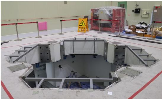
Fig. 9 Top view of seismic mass
