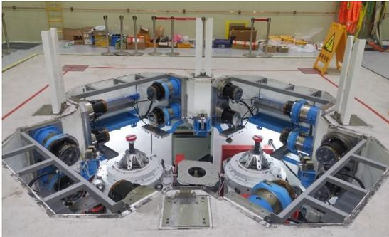
Fig. 26 Vertical shaker system before installation of H/E
