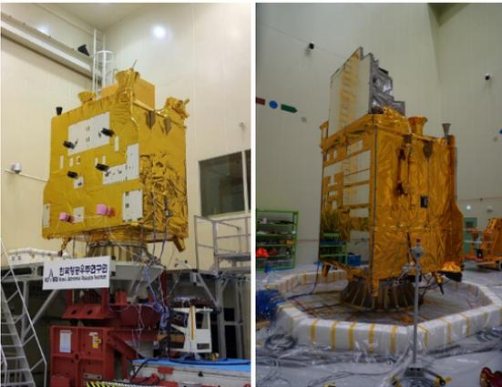
(a) Single shaker system (b) Large vertical shaker system
