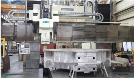
Fig. 13 Machining process for head expander
