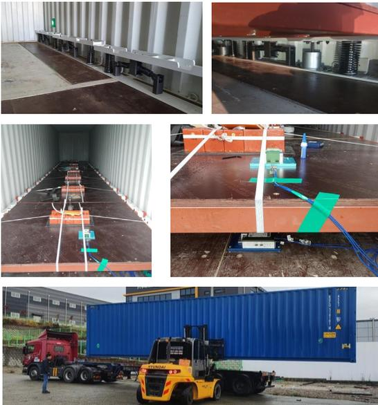
Fig. 14 Vibration measurement situations of MSNS mounts in road transport
