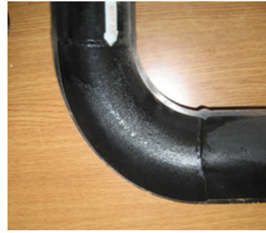
Fig. 18 Picture of a piping section thinned for 18 years in the secondary system of nuclear power plant
