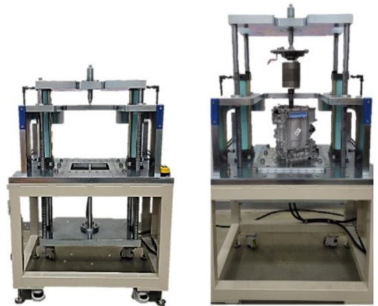
Fig. 1 Equipment for disassembling and assembling motor and reducer
