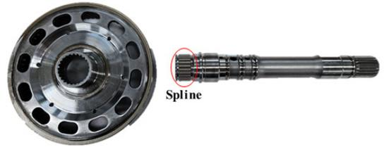
Fig. 5 Separation structure input shaft
