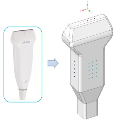
Fig. 4 Ultrasound probe modeling
