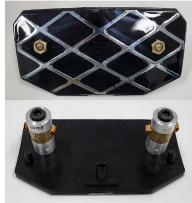
Fig. 11 Radar sensor cover assembled with 3035-4Z transducer for ultrasonic deicing test
