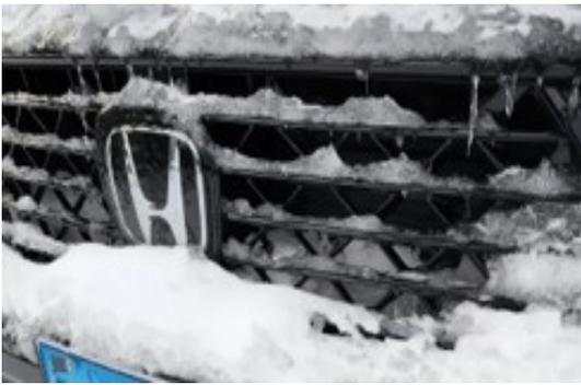
Fig. 1 Freeze of radar sensor cover
