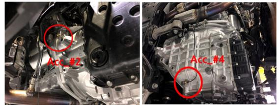
(c) Accelerometer\_#2 position
