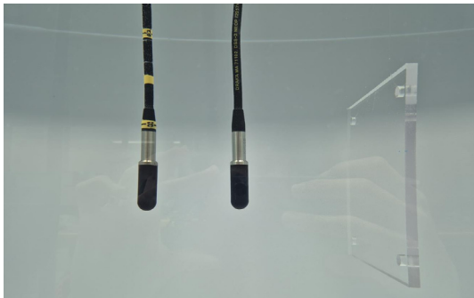
Fig. 4 Acoustic sensors and plate arrangement in the simple water tank
