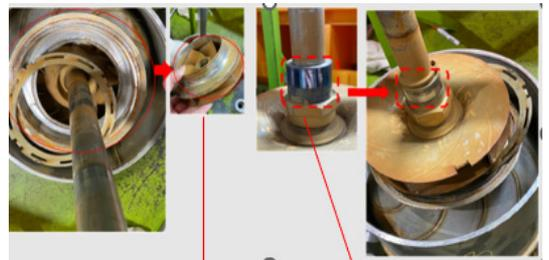
Fig. 9 Impeller friction and poor fastening
