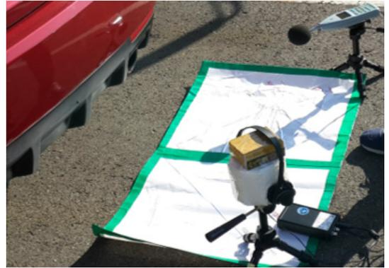
(a) Actual setup showing the measurement microphone placed behind the vehicle, capturing noise levels directly
