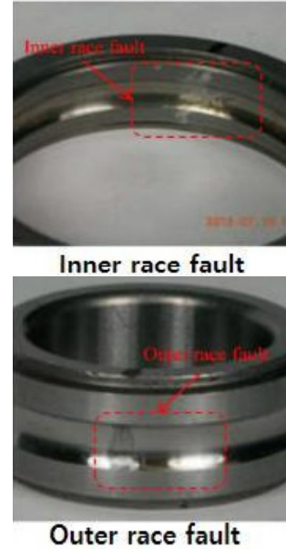
Fig. 9 Inner race fault and outer race fault(MFPT)
