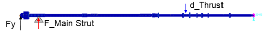
Fig. 6 Shock in the bending direction and resultant bearing(main strut bearing) reaction force and displacement
