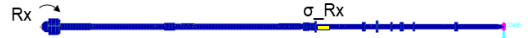
Fig. 8 Shock in the torsional direction and resultant stress on the stern tube shaft
