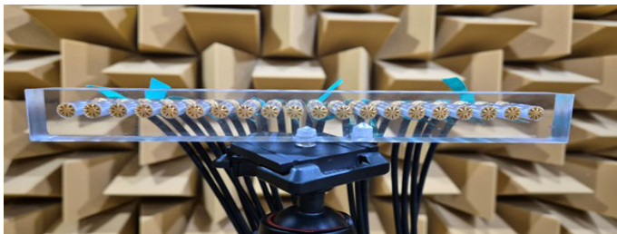
(b) Detailed view of ULA ( M = 20, d = 0.01 m)
