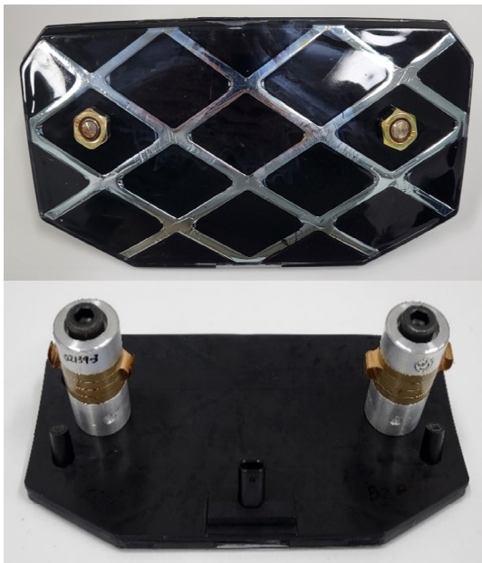
Fig. 1 Radar sensor cover sample assembled with transducers
