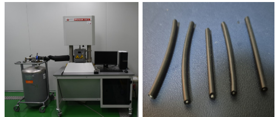
Fig. 5 DMA equipment and test specimens
