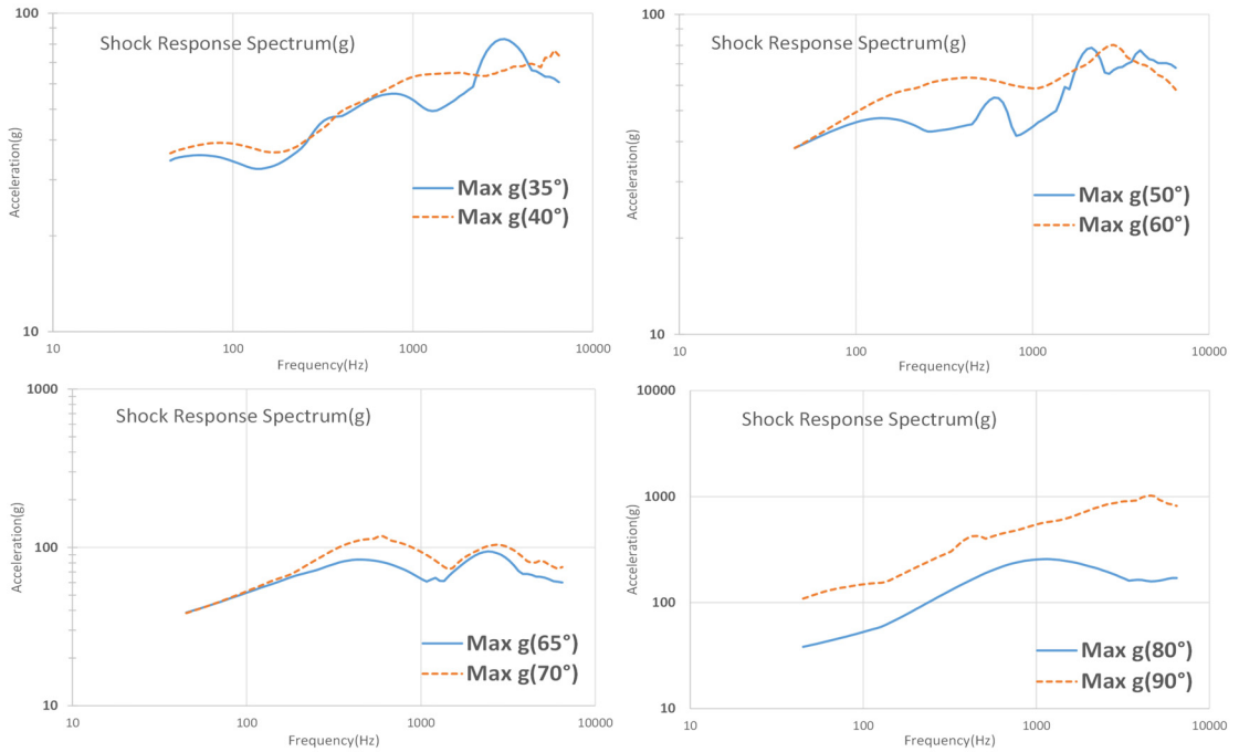
Fig. 13 Nose shock-response-spectrums by entry angle
